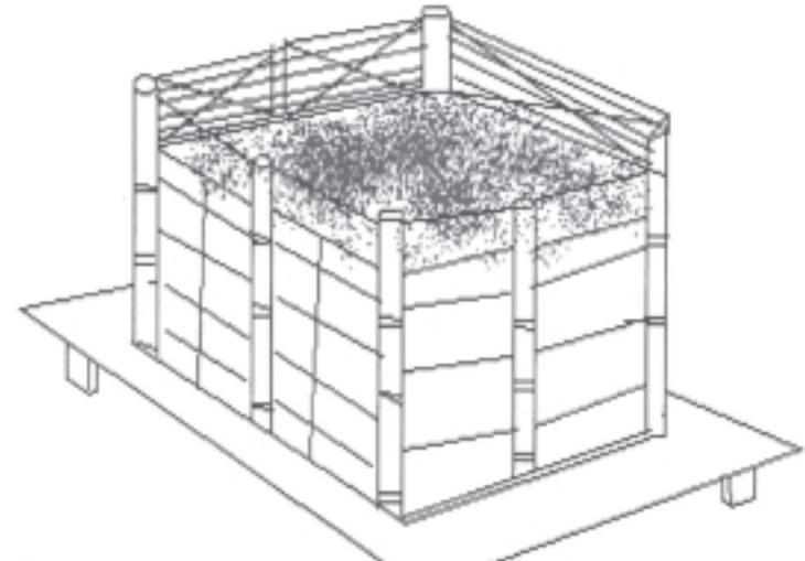
The cement-plastered bin shown above can act as a hermetic seal if a lid is properly attached to it.
